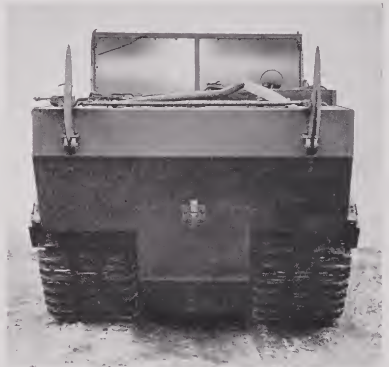
FIGURE 56. Rear view of M-29C Weasel, showing stern cell and rudders lifted.
